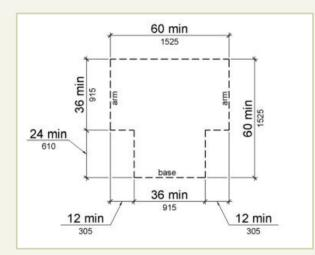
When planning for an accessible pathway, keep in mind the need for adequate turning space.
